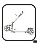
Loosen the upper lock, press the spring button and push down the T-bar to the lowest height.
