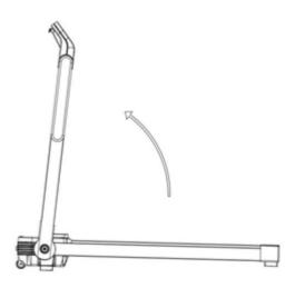
2. Raise the standpipe or Meter Asy and turn it to the direction as the arrow shows , until It stands still .
