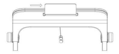
7. The illustration that guides how to use mobile holder correctly ( push the holder to the right side until it is free from the slot and turn it downwards when dismantlement needed ) .
