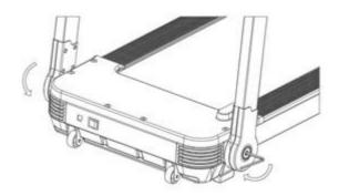
3. Take out the inner hexagon spanner(#6) from spare kit, put one end of the spanner into the screw hole of decorative cover ,tighten the screw in clockwise direction. the same installation method to the other end .(Loosen the screws in anticlockwise direction when dismantlement needed).
