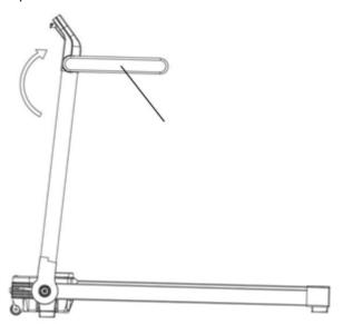
4. Keep the handrails in place as the arrow direction to adjust after the standpipe installation work finished .
