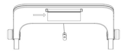
6. Turn the mobile holder upward after pushing the mobile holder to the right side ( as the arrow shows ) until the holder is free from the slot.
