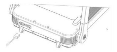
8. Keep the plug in the right socket , Orange light will be on when press the switch to "-" position.
