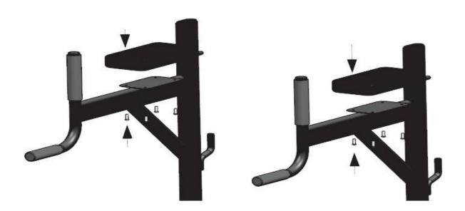
Step 7: Installing the back cushion
