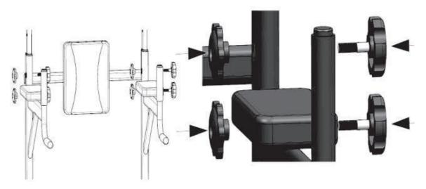
Step 11: Installing sit-up board
