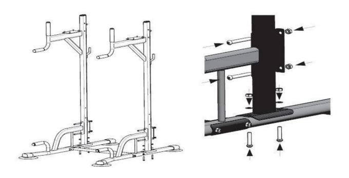
Step 5: Install the reinforcement tube
