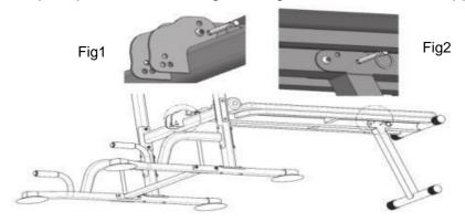
Step 14: Installing the footrest assembly
