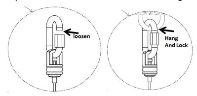
Step 3: Adjust the wire cable's length.
