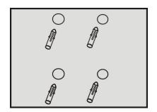
d. Fasten the four ST4\*35mm screws into the plastic expansion screws one by one, make the 4-5mm of screws higher than metope. (As shown below)
