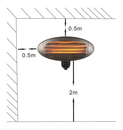
H.For the safe use of the product, please install the product in correct installation method, never install the product inversely on the wall or be fixed on the ceiling. (As shown below)
