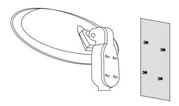
F.In order to meet customer needs, the head of the product can be move up and down for 45-degree angle. (As shown below)
