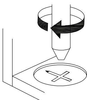
**EN**\_ Turn cam lock clockwise to tighten.
