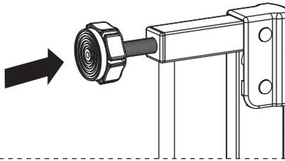
Insert the threaded spindle rods with adjustment wheels into the hole on all four corners of the sides of the gate. (Figure 2-1)
