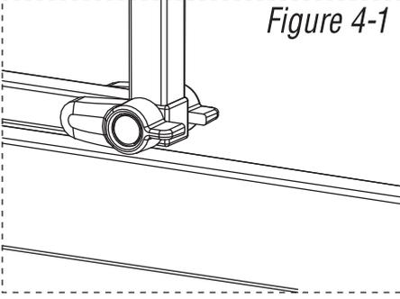
**To Open** - Ensure that the base locks at the bottom of the gate door are in the horizontal position, (Figure 4-1) then slide the top and bottom levers toward the door and swing open. (Figure 4-2)
