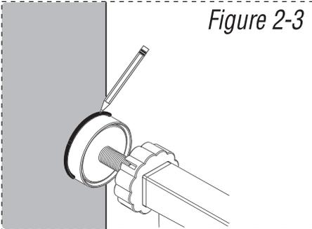
Once you are satisfied with the placement of your gate trace the spindle rods rubber feet onto the surface of your opening making sure these are level (Figure 2-3). Then remove the gate from the opening. Then screw the 4 wall cups to the wall using the screws (Figure 2-4), or paste the 4 wall cups using the stickers provided (Figure 2-5).
