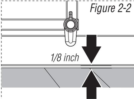
Place the gate in desired opening with the bottom close to the floor. The distance between the bottom of the gate and the floor should be less than 1/8 inch (Figure 2-2).
