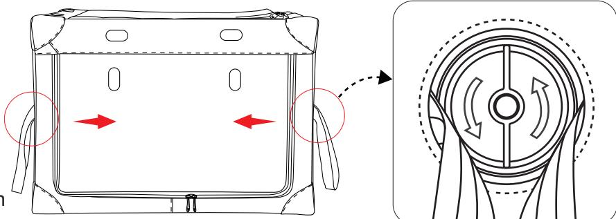
**EN\_3.2Open the magic tape on four tubes of the pet cage.**
