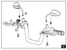
3. using 4pcs 4x12 screw to tighten.
