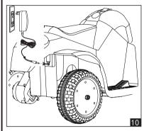
10. Battery charge: please charge tricycle when battery is low. Charging hole is on the left side of the right wheel. Connecting charging hole, then charge(10). (Notice: cannot play when charging, charging only under adult supervision)
