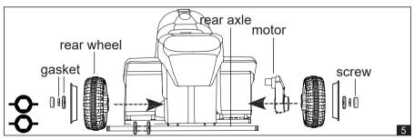
5. Assembling order to rear axle for left side is rear wheel, rear wheel cover, gasket, screw, for right side is motor, rear wheel, rear wheel cover, gasket, screw.
