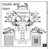
8. Inserting headstock on the front fork(1), using 4pcs 4x16 screw to tighten.
