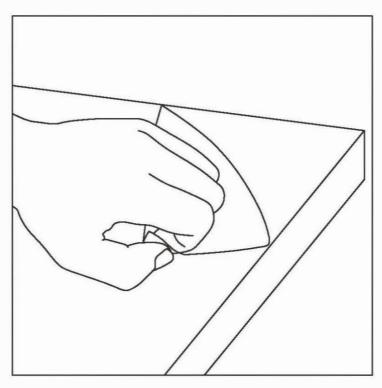
ONCE FILM IS REMOVED FULLY INSPECT ALL PARTS BEFORE YOU START ASSEMBLY
