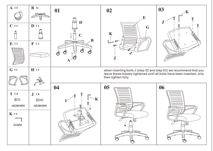
**Notes for installation:** Place **ALL** screws into the appropriate position and then tighten. **DO NOT** place and tighten one by one. If the chair comes with plastic caps, place over screws to cover holes.
