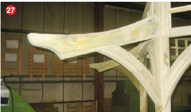
27 Secure the bearer support as shown using 2 x 50mm screws
