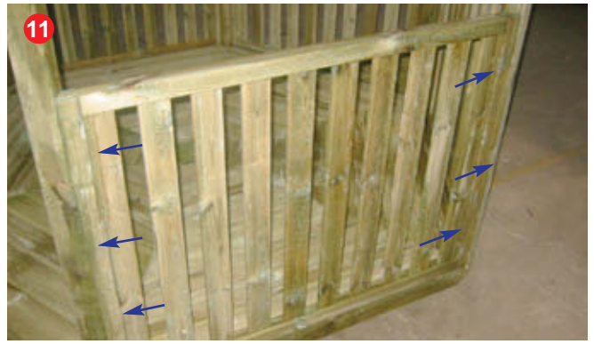
10 Sit the large fence on the floor between the uprights and secure with 6 x 70mm screws. It may help to drill pilot holes in the end frames of all the fence.
